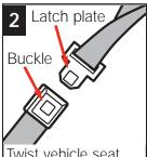
Twist vehicle seat belt and latch plate (or buckle) the buckle plate over. If the buckle slides, turn the buckle. Refasten the vehicle lap belt. The release button should face out after twisting so that it is easy to reach in an emergency.
